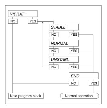
Depending on its location, the scale can be subjected to a lesser or greater extent to vibrations which are impossible to prevent. If this is the case, the program block VIBRAT offers the possibility to match the scale to the local vibrations.
