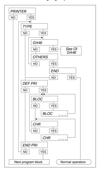
This block appears only if a serial interface is installed. In the program block you select the printer and configure the printout.
