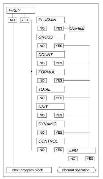
In this program block you can assign one of the following functions to the  $\rightarrow$ Fe key:
