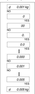
The resolution shown in the display does not correspond to the desired value. Reply with NO.
