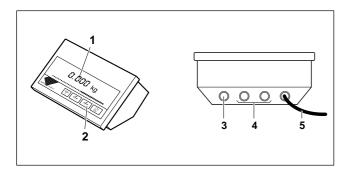
The weighing terminal comprises the following components:
