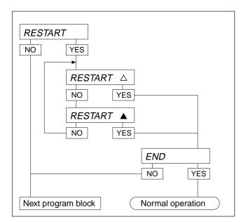
If the restart function has been activated, the zero point and tare value remain stored when the terminal is switched off. On switching on, in this case the scale shows the current weight and not zero.
