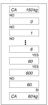
The maximum capacity shown in the display does not correspond to the desired value. Reply with NO.
