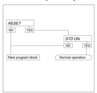
The program block RESET allows you to reset any parameters changed in the master mode to the default or standard factory settings at a keystroke.
